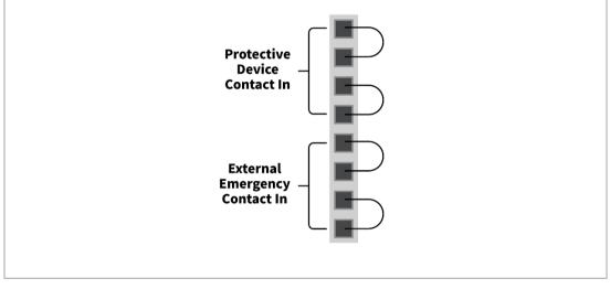
The external safety device signal recognized by the safety controller depending on the normally closed contact status, where all four contact inputs are normally closed, is as follows:
