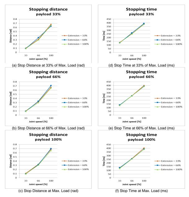
Figure C.2: Stop Distance and Stop Time of Joint 2 (Shoulder)
