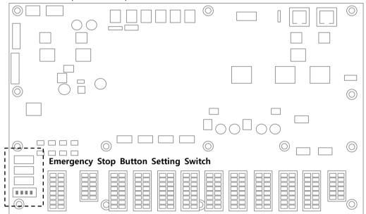
Configure the setting according to the components as follows. Upon first receiving, the setting is configured as Case 1.
