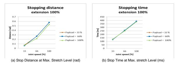
Figure C.3: Stop Distance and Stop Time of Joint 3 (Elbow)
