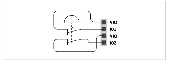
Connecting a light curtain (voltage signal) as a safety input terminal (common ground)
