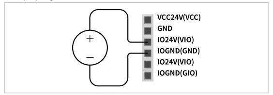
When VIO power is supplied, the IOPW (green) LED on top of the TBPWR lights up.
