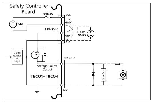
• If a negative common & sink type input device is connected
