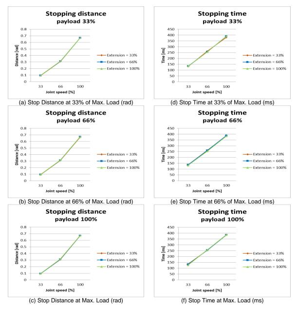
Figure C.1: Stop Distance and Stop Time of Joint 1 (Base)
