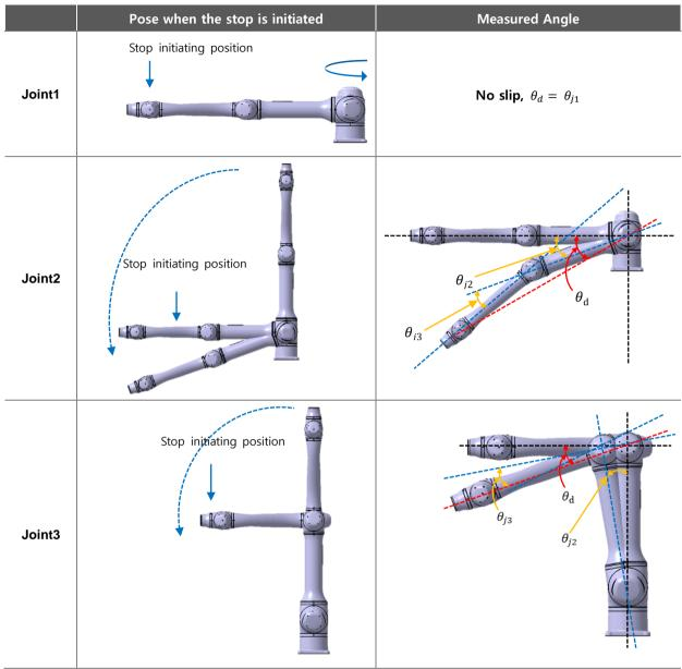
Table C.2 the pose when the stop is initiated and the measured angle  $(\theta_d)$
