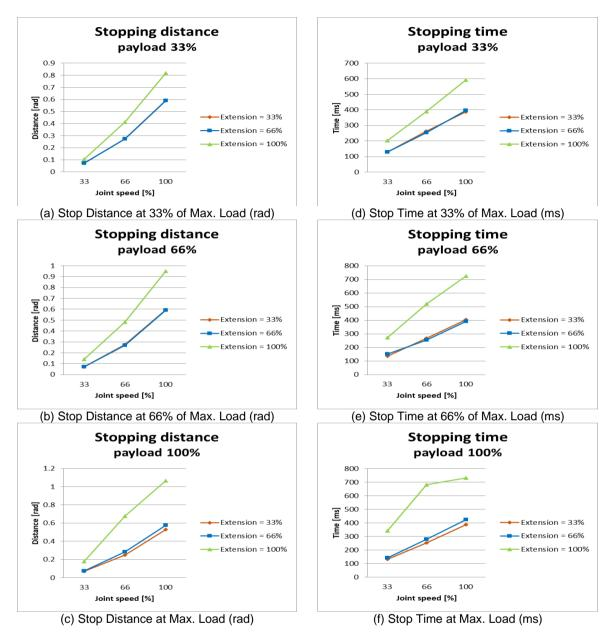
Figure C.5: Stop Distance and Stop Time of Joint 2 (Shoulder)
