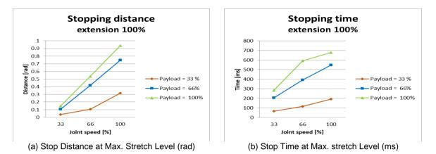
Figure C.6: Stop Distance and Stop Time of Joint 3 (Elbow)
