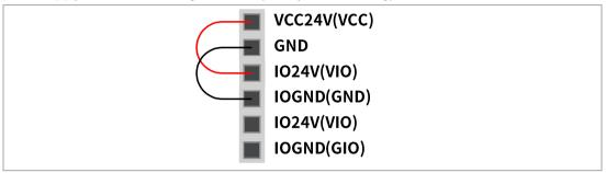
If a current greater than 2 A is required, It will be necessary to connect a separate external power source (24V) using VIO and GIO terminals.
