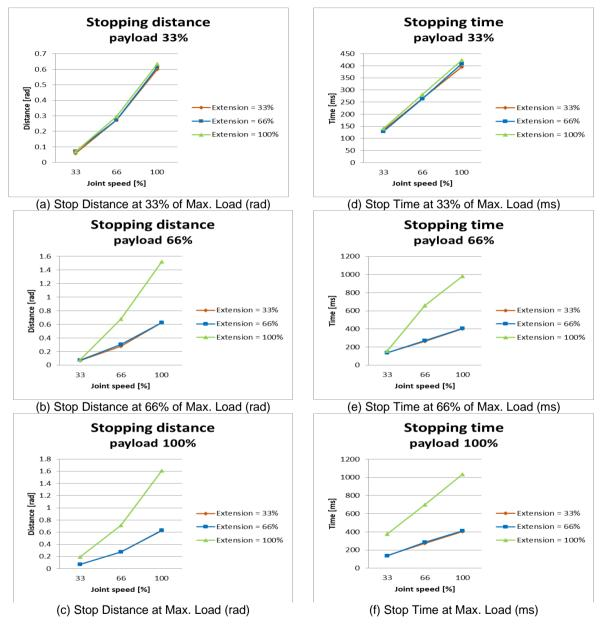
Figure C.4: Stop Distance and Stop Time of Joint 1 (Base)
