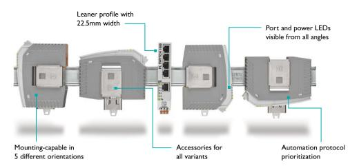
While most industrial applications use traditional DIN rail-mounting, there are many situations where depth or cable direction within a cabinet is critical. The FL SWITCH 1000 series offers 5 different mounting options to cover just about every application. Regardless of how the switch is mounted, you can be informed of the switch status with diagnostic LEDs that are visible from any angle.
